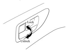
To lock either front door with the doorlock knob from the outside, push the door-lock knob to the lock position and close the door (pulling the door handle is not required).
